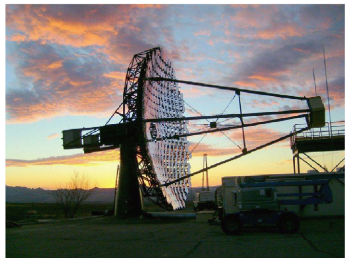
Fig. 1. Side view of one of the VERITAS telescopes showing the camera box at the focal point of a 12-m-diameter tessellated reflector of the Davies–Cotton design and balanced by a counterweight behind the reflector.
