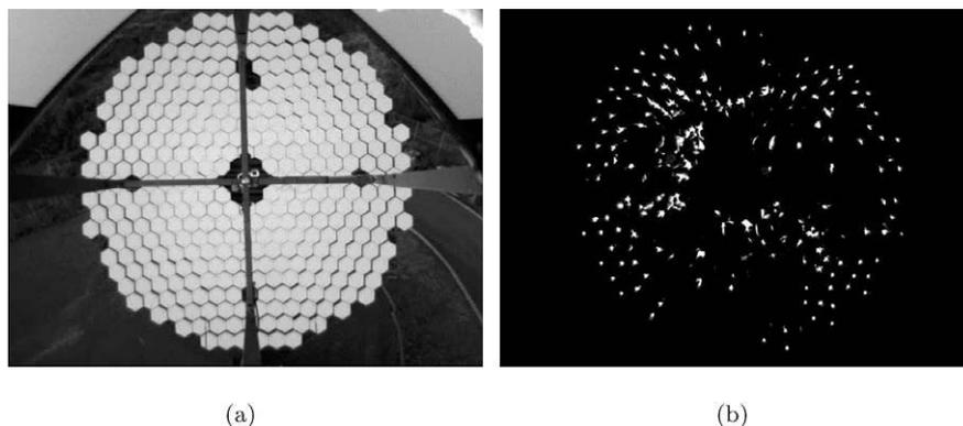
**Fig. 3.** Images, taken by the digital camera, of one of the VERITAS reflectors during the day (a) and at night while pointing at a star (b). The bright spots in the right-hand panel are caused by starlight reflecting off well-aligned facets while the dark regions indicate poorly-aligned facets.
