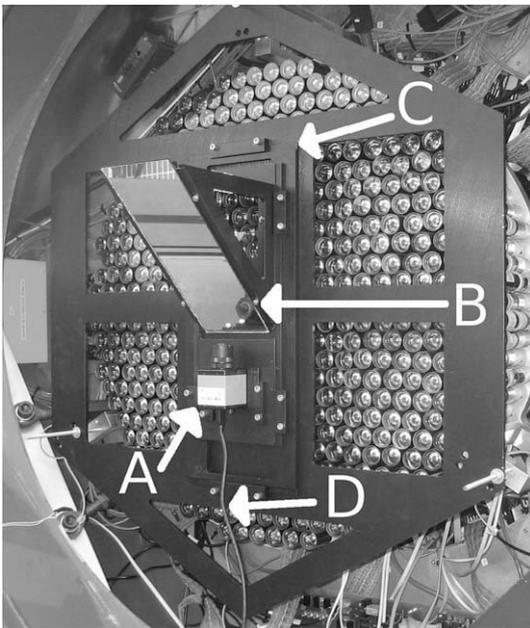
**Fig. 2.** A photograph of the alignment apparatus mounted on one of the VERITAS PMT cameras. Arrow A indicates the digital camera; B, the 45° mirror; C, the x-y positional stage and D the cable connecting to the data acquisition notebook computer (not shown).
