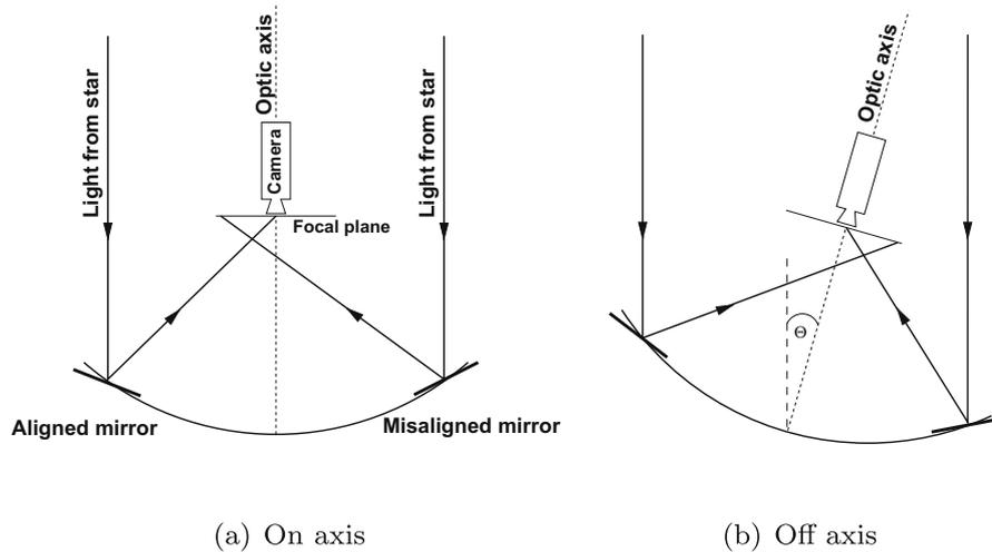
**Fig. 1.** An illustration of the raster scan method. In panel (a) the well-aligned facet will appear bright in the CCD-camera image while the mis-aligned facet will be dark. In panel (b) the mis-aligned facet will appear brightest when the angle between the star and the telescope pointing direction,  $\theta$ , is twice the mis-alignment angle of the facet.
