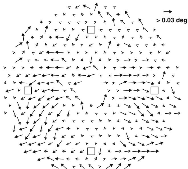
**Fig. 5.** A mis-alignment map for one of the VERITAS telescopes. The length of the arrow indicates the size of the mis-alignment of an individual facet. Mis-alignments angles greater than  $0.03^\circ$  are not drawn to scale and are plotted with a solid arrow head. The black squares indicate the position of the quadrupod arms of the telescope.
