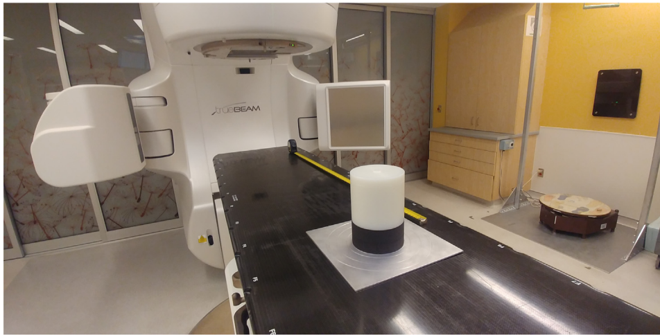
Fig. 3. The passive NNS positioned at the location of measurement in our radiotherapy bunker. The black material underneath the NNS is a foam base used to maintain the central He-3 detector at a constant height.
